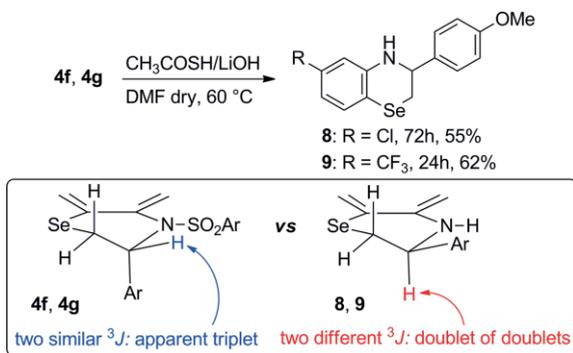
Scheme 3. Synthesis of *N*-unsubstituted benzoselenazines **8** and **9** and the conformational consequences of substitution on nitrogen of the selenazines.
