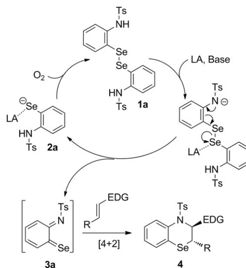
Scheme 1. Synthetic one-pot procedure for the preparation of benzo[*b*][1,4]selenazines **4** from the parent 2-*N*-sulfonylaminoaryl diselenide (**1a**). EDG = electron-donating group; LA = Lewis acid.
