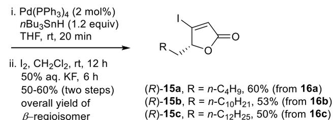
Scheme 2. Synthesis of  $\beta$ -iodo-butenolides **15**.
