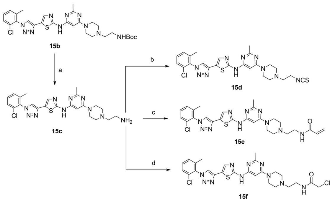
**Scheme 3.** Reagents and conditions: (a) TFA, CH<sub>2</sub>Cl<sub>2</sub>, r.t., 80%; (b) DCC, CS<sub>2</sub>, CH<sub>2</sub>Cl<sub>2</sub>, r.t., 41%; (c) acryloyl chloride, Et<sub>3</sub>N, CH<sub>2</sub>Cl<sub>2</sub>, r.t., 47%; (d) chloroacetyl chloride, Et<sub>3</sub>N, CH<sub>2</sub>Cl<sub>2</sub>, r.t., 37%.
