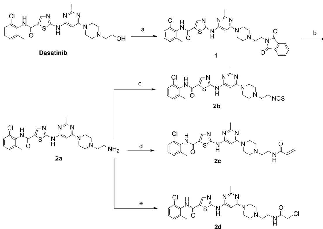
**Scheme 1.** Reagents and conditions: (a)  $\text{PPh}_3$ , phthalimide, DIAD, THF, r.t., 88%; (b)  $\text{N}_2\text{H}_2\cdot\text{H}_2\text{O}$ , EtOH, 78 °C, 72%; (c) DCC,  $\text{CS}_2$ ,  $\text{CH}_2\text{Cl}_2$ , r.t., 52%; (d) acryloyl chloride,  $\text{Et}_3\text{N}$ ,  $\text{CH}_2\text{Cl}_2$ , r.t., 49%; (e) chloroacetyl chloride,  $\text{Et}_3\text{N}$ ,  $\text{CH}_2\text{Cl}_2$ , r.t., 55%;
