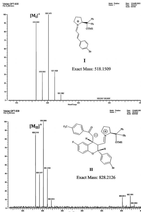
Figure 4. The HRMS spectra of the intermediates **I** (top) and **II** (bottom).
