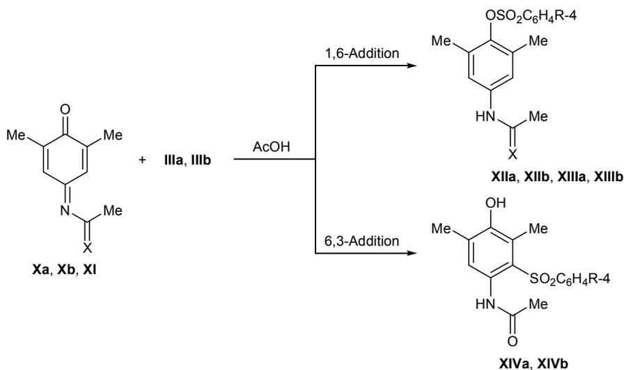
**X**, X = 4-MeC<sub>6</sub>H<sub>4</sub>SO<sub>2</sub>N (**a**), 4-ClC<sub>6</sub>H<sub>4</sub>SO<sub>2</sub>N (**b**); **XI**, X = O; **XII**, R = Me, X = 4-MeC<sub>6</sub>H<sub>4</sub>SO<sub>2</sub>N (**a**), 4-ClC<sub>6</sub>H<sub>4</sub>SO<sub>2</sub>N (**b**); **XIII**, X = O, R = Me (**a**), Cl (**b**); **XIV**, R = Me (**a**), Cl (**b**).
