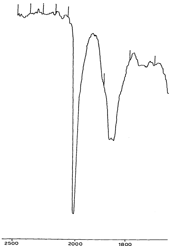
Fig. 2. Infrared spectrum of [(Ph_3P)_2N]_2[Rh_{14}(CO)_{26}] in acetone.
