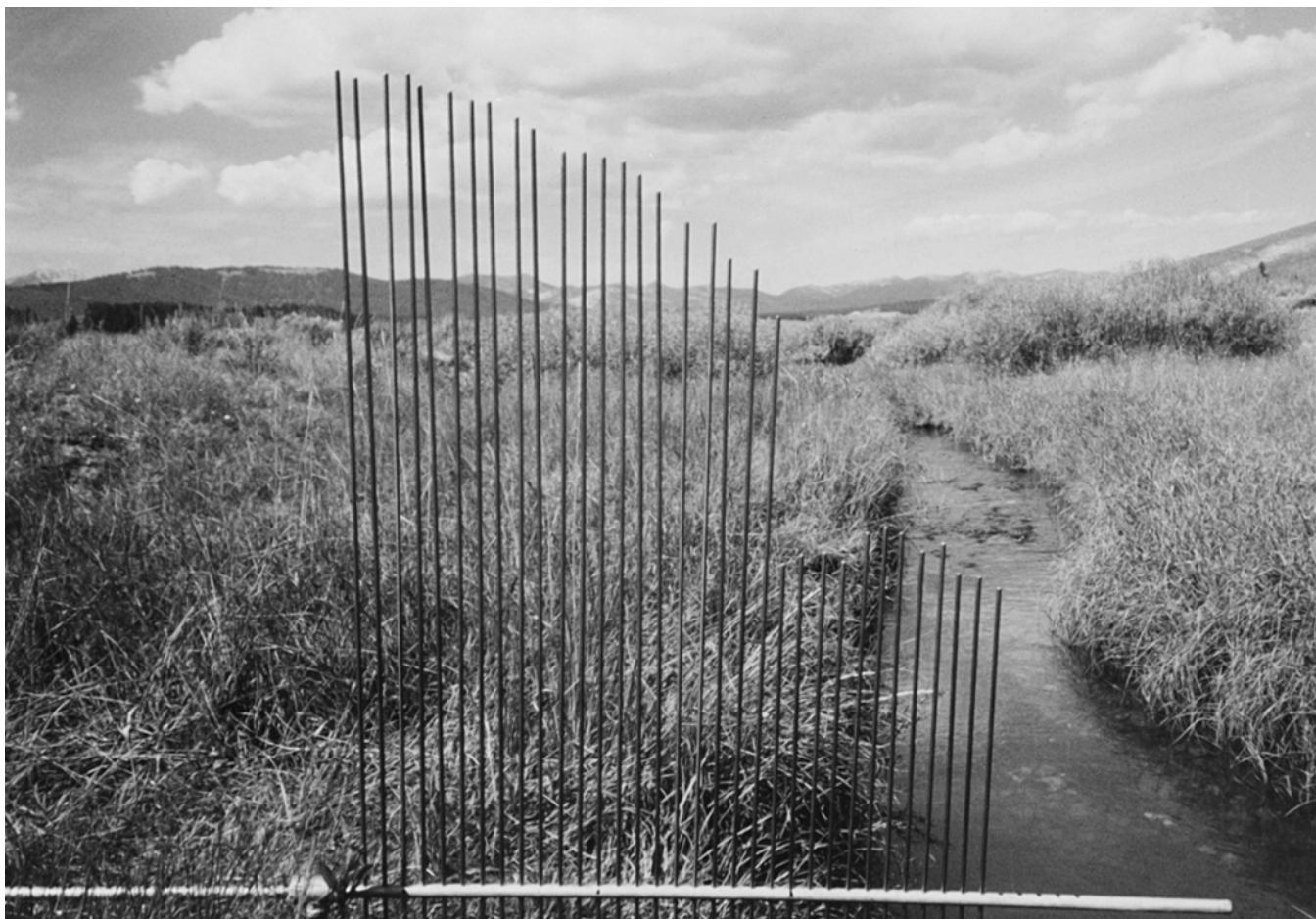
Figure 1. Bankometer positioned on a study plot in central Idaho.
