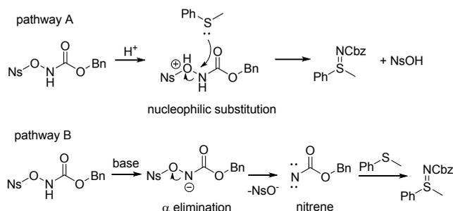
**Scheme 4.** Proposed mechanism for the imidation of thioether.
