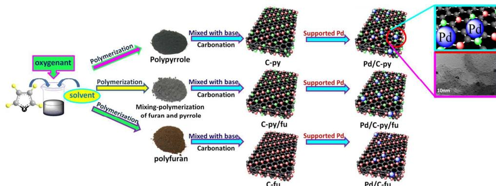
**Scheme 1.** Preparation of Pd/C-py, Pd/C-py/fu and Pd/C-fu through the palladium nanoparticles supported on functionalized porous carbons
