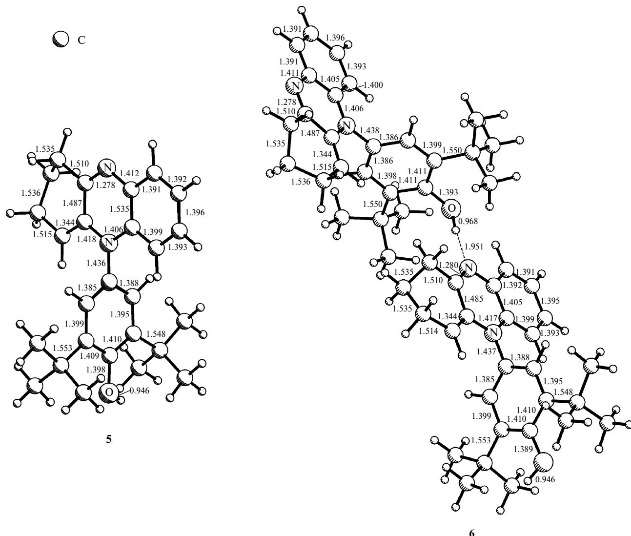
**Fig. 3.** Geometric characteristics and the minimum harmonic vibrational frequencies ( $\omega_1$ ) of monomer **5** and dimer **6a** calculated at the RHF/LanL2DZ level. The bond lengths are given in Å. For compound **5**,  $\lambda = 0$  ( $\omega_1 = 19.9 \text{ cm}^{-1}$ ); for compound **6**,  $\lambda = 0$  ( $\omega_1 = 5.6 \text{ cm}^{-1}$ ),  $E_{\text{complex}} = 7.8 \text{ kcal mol}^{-1}$ .
