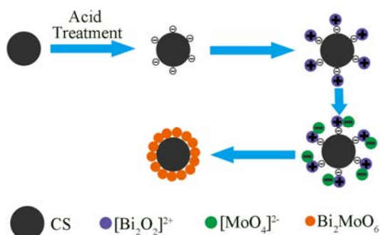
Fig. 2 Schematic illustration of the growth process of CS@BMO composite.
