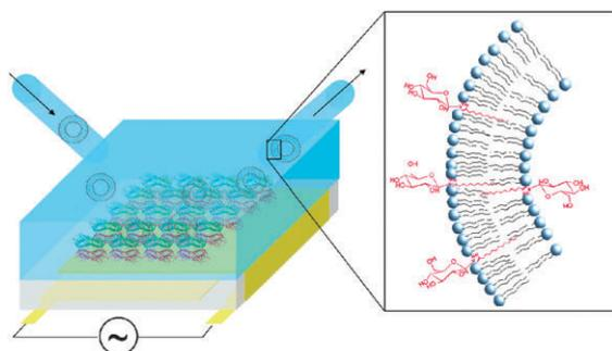
**Fig. 1** Con A layers exposed to functionalised vesicle solutions within a QCM system.
