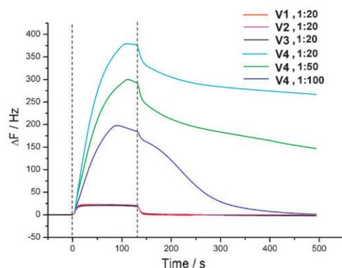
**Fig. 2** QCM adsorption profiles for alkyl glycoside functionalised vesicles at different molar ratio of alkyl glycosides **1–4** to phospholipids (1 : 20/mol : mol = 10  $\mu\text{M}$  in glycoside).
