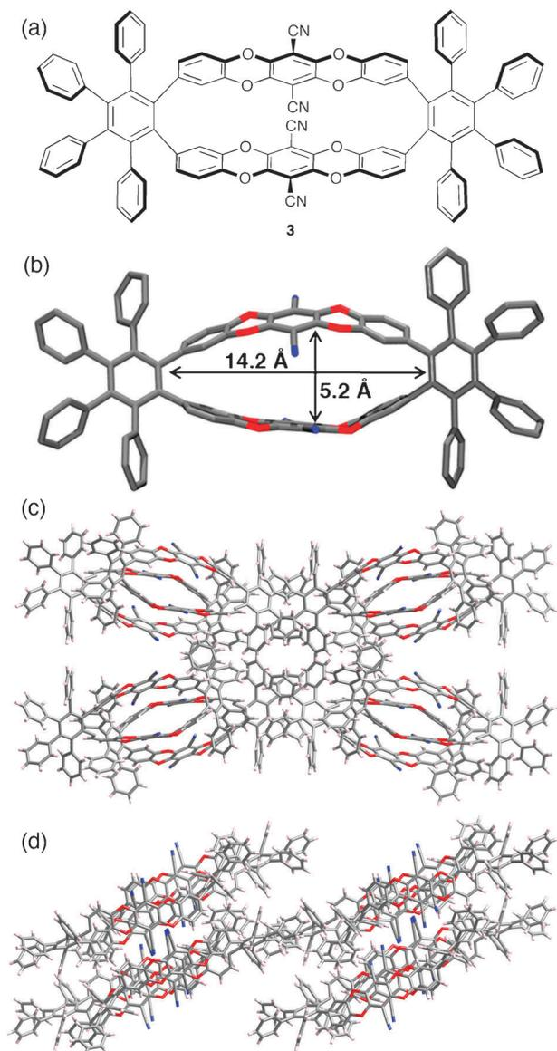
**Fig. 1** (a) The molecular structure of **3** and (b) its structure from a single crystal X-ray diffraction study. The packing of **3** viewed along (c) the *z*-axis and (d) the *y*-axis of the crystal showing the channels that are filled with disordered solvent.
