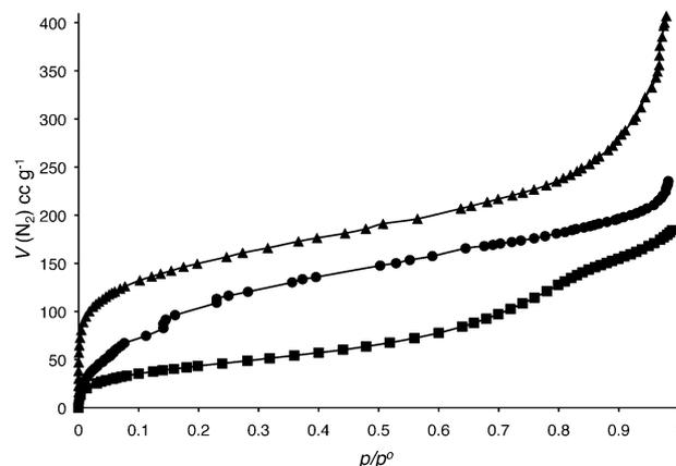
**Fig. 2** Nitrogen adsorption isotherms for **3** (■); HPB-PIM-1 (●) and HPB-PIM-2 (▲).
