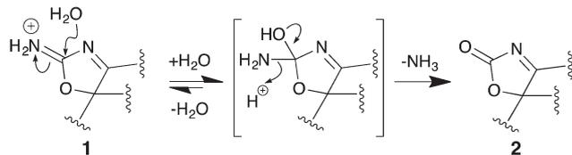
Fig. 5 Mechanism for hydrolysis of 1 to 2.
