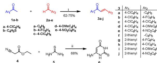
Scheme 1: Reagents and conditions: (i) KOH, methanol, rt, (ii) NaOEt/ethanol, reflux, 4 h.
