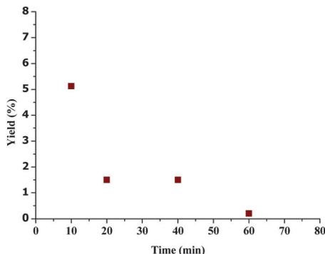
Fig. 6 Zn-porphyrin yield vs. reaction time (min). MW enhanced reactions carried out in dioxane in the presence of  $\text{Zn}(\text{AcO})_2$  (0.13 M), 50 bar ( $\text{N}_2$ ), 140 °C, reactant concentration 0.4 M.
