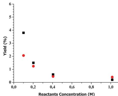
Fig. 4 Porphyrin yield vs. reactant concentration. MW enhanced reactions carried out in dioxane, 50 bar (N<sub>2</sub>), 20 min, 140 °C (red circle) and 170 °C (black square).
