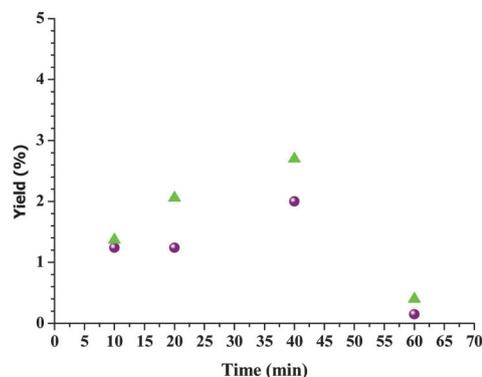
Fig. 5 Porphyrin yield vs. reaction time (min). MW enhanced reactions carried out in dioxane, 50 bar (N<sub>2</sub>), 140 °C, 0.1 M (green triangle) and 0.2 M (purple sphere).
