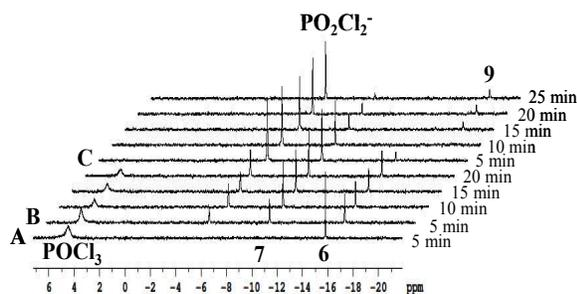
Figure 1. <sup>31</sup>P NMR spectra for the synthesis of **5l**.
