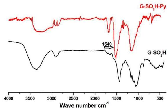
**Fig. 3** FT-IR spectra of G-SO<sub>3</sub>H and G-SO<sub>3</sub>H-Py
