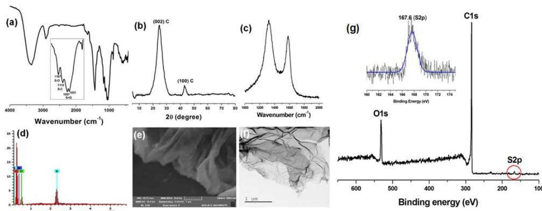
**Fig. 1** a) FT-IR, b) PXRD, c) FT-Raman spectrum, d) EDS, e) SEM image and f) TEM Image, g) XPS of G-SO<sub>3</sub>H
