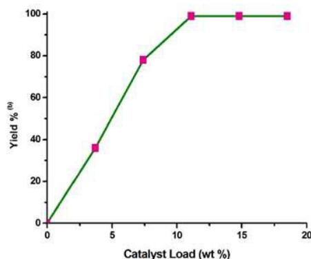
Fig. 2 Catalyst load optimization (<sup>b</sup> isolated yield)
