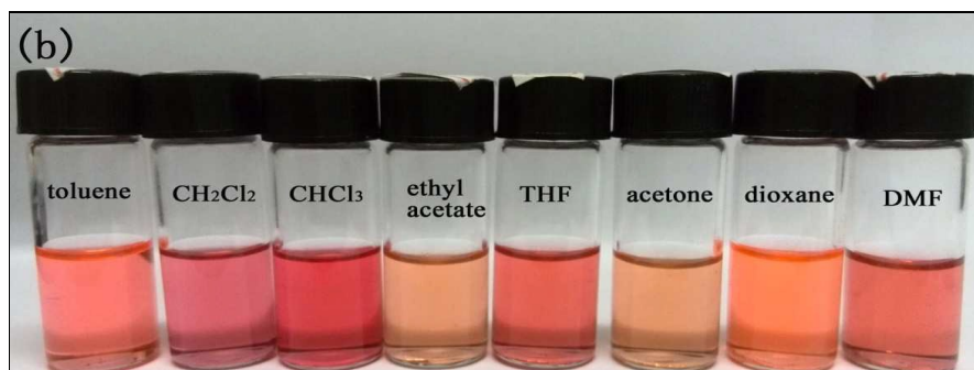
Fig. 2. (a) The normalized UV-vis spectra and (b) photographs of N1 in different solvent.
