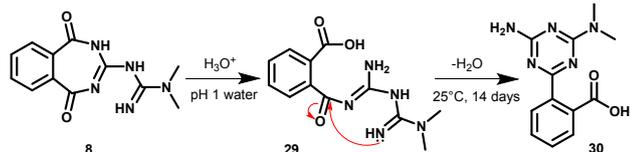
**Figure 5.** Degradation pathway of compound **8** in acidic water. After 1 day, almost full hydrolysis to acid **29** is observed. Then slow cyclodehydration to triazine **30** occurred (25% conversion after 14 days)
