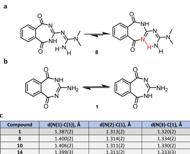
**Figure 4.** Structure and tautomers in solution: a). Compound **8** offers an intramolecular H-bonding possibility that congeals the equilibrium toward one tautomer and breaks the symmetry of the molecule b). Compound **1** is in permanent equilibrium between two tautomer forms and displays symmetric signals in  $^1\text{H}$  NMR. c). C-N bond lengths of the guanidine within compounds **1**, **8**, **10** and **14** in crystal solid state.
