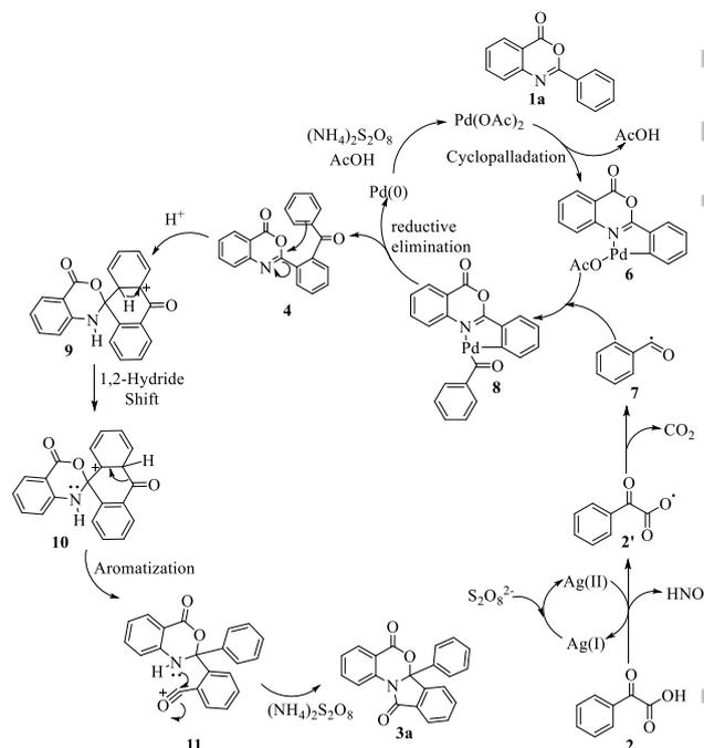
**Scheme 3.** Plausible reaction mechanism.
