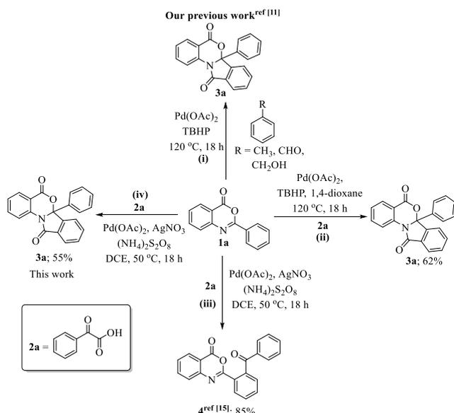
**Scheme 1.** Preliminary studies and functionalization of 2-phenyl-4*H*-benzo[*d*][1,3]oxazin-4-one with  $\alpha$ -oxocarboxylic acid.
