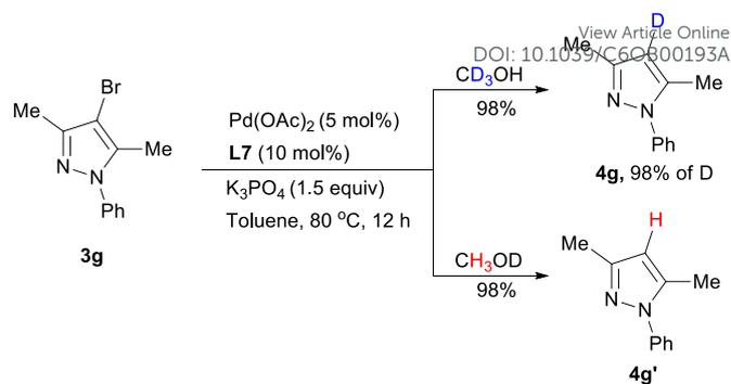
**Scheme 2.** Deuteration of 4-Bromopyrazole **3g** with CD<sub>3</sub>OH & CH<sub>3</sub>OD
