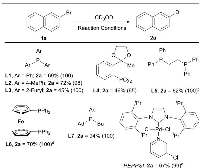
[a] Reaction Conditions: 2-Bromonaphthalene (0.5 mmol), Pd(OAc)<sub>2</sub> (5 mol%), **L1 - L4**, **L7** (10 mol%), Cs<sub>2</sub>CO<sub>3</sub> (0.75 mmol), CD<sub>3</sub>OD/Toluene (1:4), 80 °C, 12 h; [b] Conversions are inside the parenthesis; [c] GC yield; [d] **L5 - L6** (5 mol%); [e] Without Pd(OAc)<sub>2</sub>.
