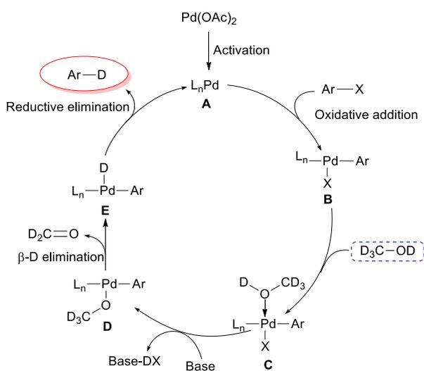
**Scheme 1.** Mechanism of Deuteration of Aryl and Heteroaryl Halides
