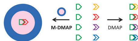
Scheme 1 Illustration of specific reaction of one substrate (from a pool of 4) using a polymeric nanoreactor as a reaction vessel (Green = 1 anhydride; yellow, red, purple and blue = 4 different alcohols).
