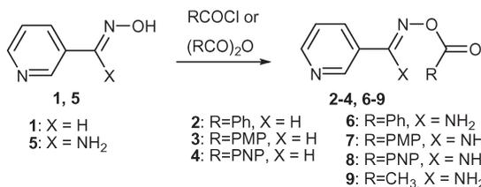
**Scheme 1** Synthesis of *meta*-pyridine derivatives **2–4** and **6–9**. Reaction conditions: acylating agent, Et<sub>3</sub>N, solvent (CHCl<sub>3</sub> or THF or DMF), 0 °C to r.t., 74–89% yield for **2–4**, 50–72% yield for **6–9** [PMP = *p*-methoxy-phenyl, PNP = *p*-nitro-phenyl].
