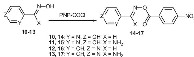
**Scheme 2** Synthesis of *ortho*- and *para*-pyridine derivatives **14–17**. Reaction conditions: PNP-COCl, Et<sub>3</sub>N, THF, 0 °C to r.t., 1.5 h, 75–88% yield.
