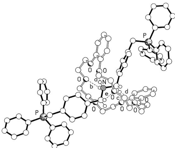
Figure 3. The cationic portion of the solid-state structure of the [2]rotaxane **4a-H** · 3PF<sub>6</sub>. The hydrogen bonding geometries, X···O, H···O [Å], and X–H···O [°]: a) 3.05, 2.26, 147; b) 2.96, 2.15, 151; c) 3.33, 2.44, 153; d) 3.21, 2.41, 156; e) 3.22, 2.33, 156.
