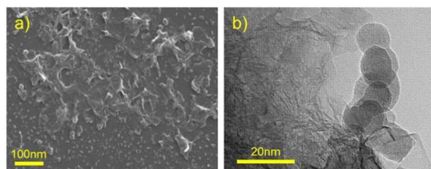
Fig. 2 a) SEM and b) TEM images of GO–CuBr nanocatalytic system.
