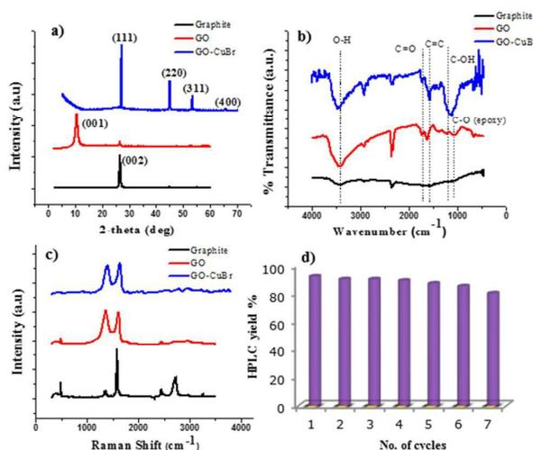
Fig. 1 a) PXRD, b) FTIR, c) RAMAN spectra of graphite, GO, and GO–CuBr, d) recycling of GO–CuBr as catalyst.
