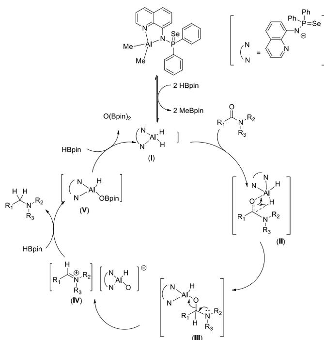
**Scheme 2.** Proposed mechanism for the selective reduction of amides to amines.
