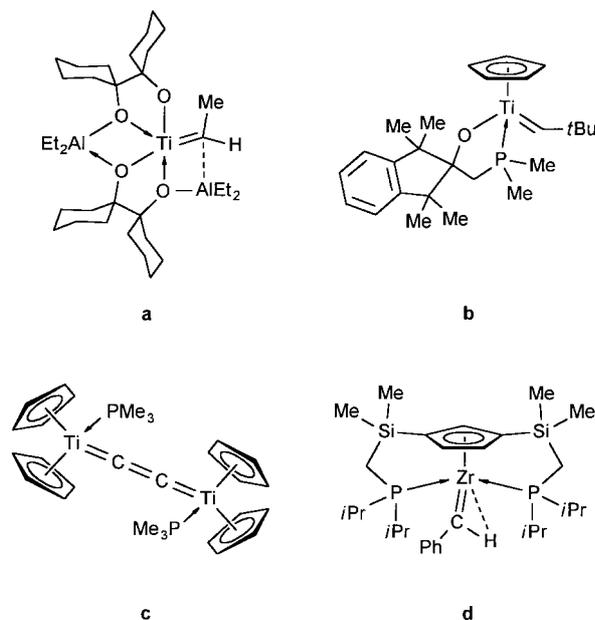
Scheme 1. Selected, structurally characterized alkylidene complexes of titanium and zirconium complexes. **a**: Ti–C 1.933(6) Å,  $\delta(\text{Ti}=\text{C}) = 202.1$  (main components);<sup>[6]</sup> **b**: Ti–C 1.911(3) Å,  $\delta(\text{Ti}=\text{C}) = 278.1$ ;<sup>[7]</sup> **c**: Ti–C 2.051(2) Å,  $\delta(\text{Ti}=\text{C}) = 258.1$ ;<sup>[8]</sup> **d**: Zr–C 2.024(4) Å,  $\delta(\text{Zr}=\text{C}) = 229.4$ .<sup>[9]</sup>
