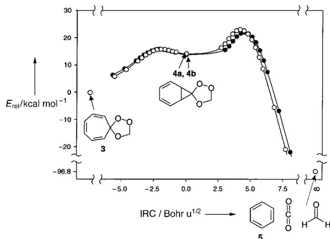
Figure 1. Relative energies  $E_{\text{rel}}$  in the course of the fragmentation of the spiroozonide **3** calculated at the B3LYP/6-31G\* level (IRC = intrinsic reaction coordinate). The values of the IRC are relative to the norcaradiene intermediates **4a** and **4b**.
