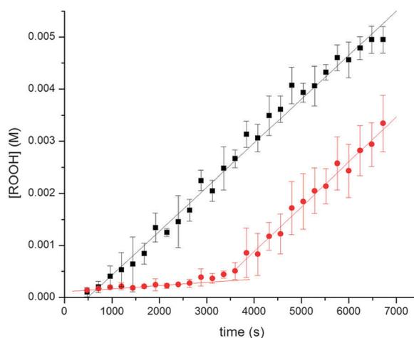
**Fig. 2** Autoxidation of 7-dehydrocholesterol (78 mM) in 1,2-dichlorobenzene initiated with 52  $\mu\text{M}$  of MeOAMVN (■), and its inhibition with 4  $\mu\text{M}$  of PMHC (●) at 37 °C.
