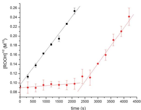
**Fig. 3** Autoxidation of neat hexadecane initiated with 8 mM TetOOH (■), and its inhibition with 1 mM of BHT (●) at 160 °C.
