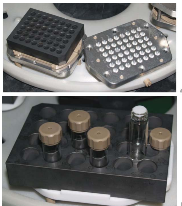
Fig. 1 (a) A 48-position silicon carbide plate; (b) A 24-position silicon carbide plate capable of holding standard glass vials.
