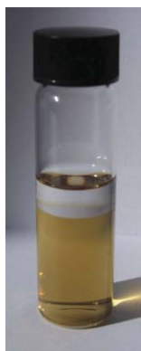
Fig. 4 Photograph of the separated phases after hydroformylation of 1-octene in the presence of [OctMim]Br ( 0.5 \text{ mol dm}^{-3} ).
