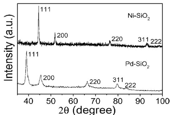
Fig. 1 XRD patterns of Ni-SiO<sub>2</sub> and Pd-SiO<sub>2</sub>.
