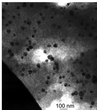
Fig. 2 TEM image corresponding to Ni-SiO<sub>2</sub>.
