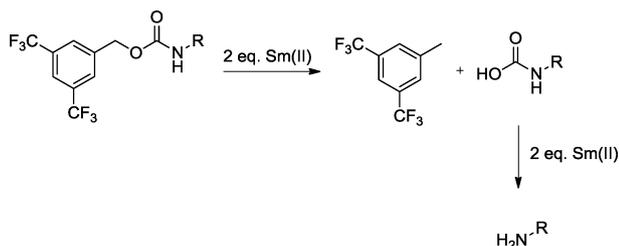
**Scheme 2** A 4-electron reduction of the carbamate bond with SmI<sub>2</sub>, R<sub>3</sub>N and H<sub>2</sub>O yields bis-CF<sub>3</sub>-toluene and the free amine.**Table 2** Stability tests performed on **1**
