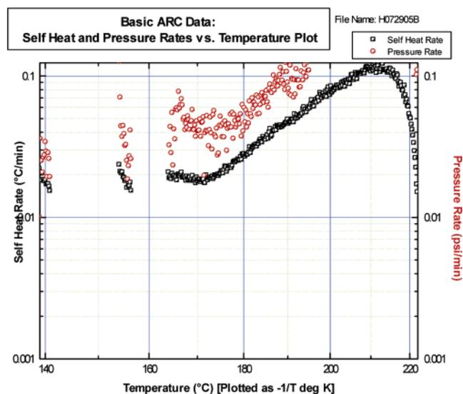
**Figure 4.** Self-heat and pressure rate exotherms observed during the ARC screening of the reaction mixture, sampled after the sodium chlorite addition.
