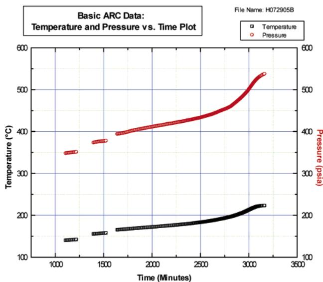
**Figure 3.** Temperature and pressure profiles for exotherms observed during the ARC screening of the reaction mixture, sampled after the sodium chlorite addition.
