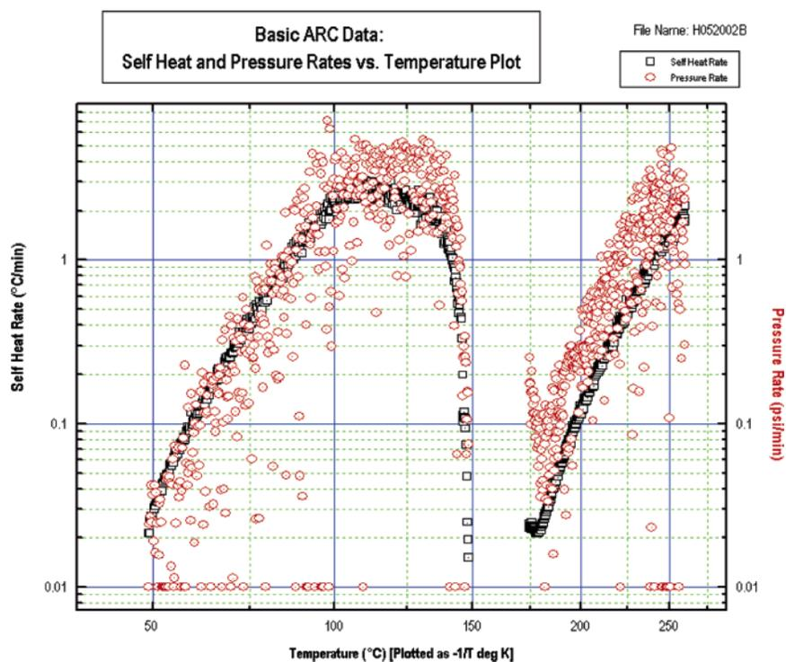
**Figure 2.** Self-heat and pressure rates for two exotherms observed during the ARC screening of the organic phase, sampled after the hydrogen peroxide addition.
