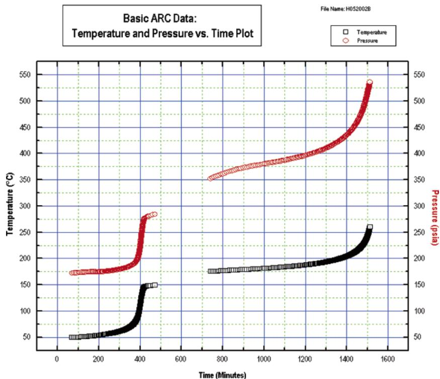
**Figure 1.** Temperature and pressure profiles for two exotherms observed during the ARC screening of the organic phase, sampled after the hydrogen peroxide addition.
