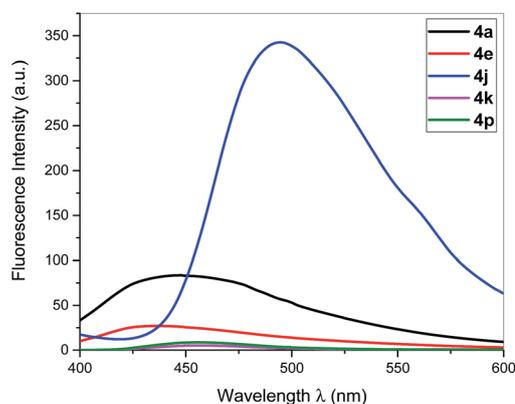
Fig. 2 Fluorescence spectra of dipyrzolylmethanes **4a**, **4e**, **4j**, **4k** and **4p** ( $1 \times 10^{-4}$  M in MeCN,  $\lambda_{\text{ex}} = 330$  nm).
