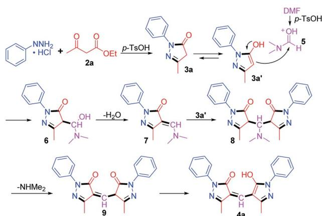
Scheme 3 Proposed reaction mechanism for the formation of **4a**.
