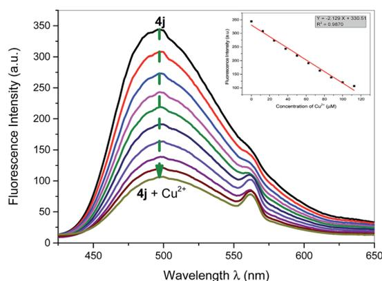
Fig. 4 Fluorescence response of dipyrzolylmethane **4j** with respect to various concentrations of  $\text{Cu}^{2+}$  ions (0–112.5  $\mu\text{M}$ ). Inset: linear correlation between the fluorescence intensity and  $\text{Cu}^{2+}$  ions.
