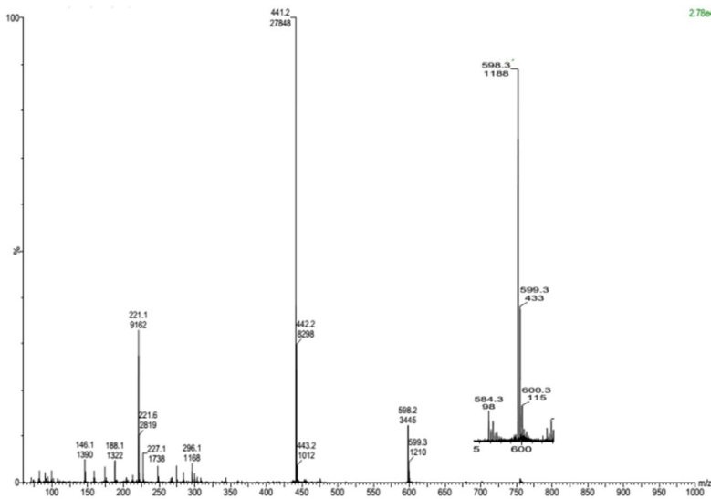
Figure 7: MS(ES+) mass spectrum of TAME5OX.
