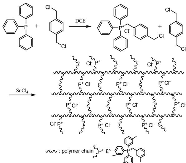
Scheme 1 The synthesis of the crosslinked polymer with IL moiety.
