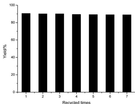
Fig. 3 The recycled catalytic activity of the polymer.
