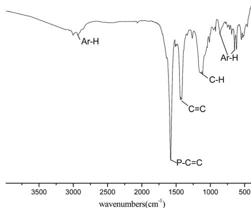
Fig. 2 The FT-IR spectrum of the polymers.
