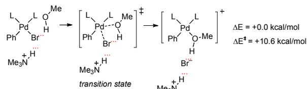
**Figure 6.** Pathways for halide ionization in methanol solvent. The B3LYP DFT functional was used in conjunction with the LanL2dz ECP basis set for Fe and Pd. The solvent effect in methanol was taken into account by IEFPCM.
