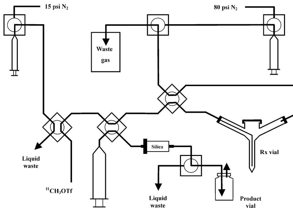
Figure 4. Radiosynthesis and SPE purification system of  $^{11}\text{C}$ -labeled edrophonium and analogues.
