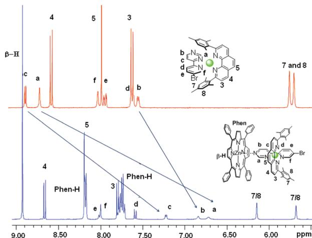
Fig. 1 (Top) <sup>1</sup>H NMR spectrum of complex **10** in CD<sub>2</sub>Cl<sub>2</sub> at 298 K. (Bottom) Complex **10** after addition of ZnTPP. The upfield shifts indicate axial coordination of **10** to ZnTPP.
