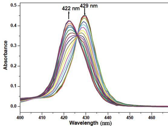
Fig. 4 UV-vis titration of  $19$  ( $1 \mu\text{M}$ ) vs.  $[\text{Cu}(5)]^+$  ( $0.1 \text{ mM}$ ) in DCM at 298 K. After 3 equivalents of copper complex addition, the intensity at 422 nm remains constant.
