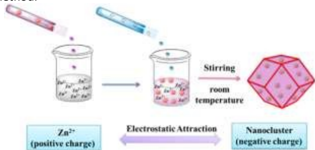
Scheme 1. Schematic illustration showing the rational encapsulation of APNCs@MOFs by Electrostatic Attraction.
