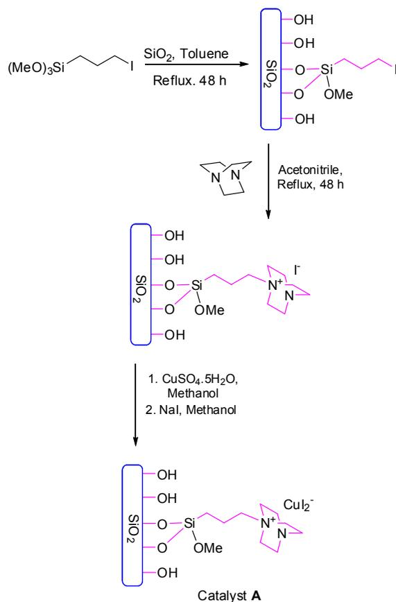
Scheme 1. Synthesis process of Cu(I)-DABCO@SiO<sub>2</sub> (catalyst A)
