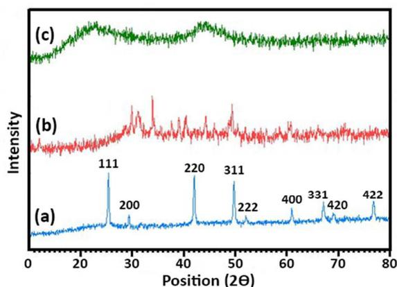
**Fig 2.** XRD pattern of the fresh catalyst **A** (a), the recovered catalyst **A** after third cycle (b) and the reactivate catalyst **A** after the treatment with NaI.
