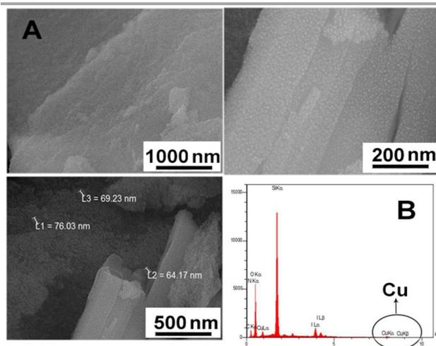
**Fig 3.** FE-SEM images and SEM-EDX spectrum of catalyst **A**.
