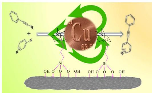
Nano-CuI stabilized in functionalized-DABCO silica matrix was prepared, characterized and evaluated as a new heterogeneous nanocatalyst in copper-catalyzed Sonogashira coupling
