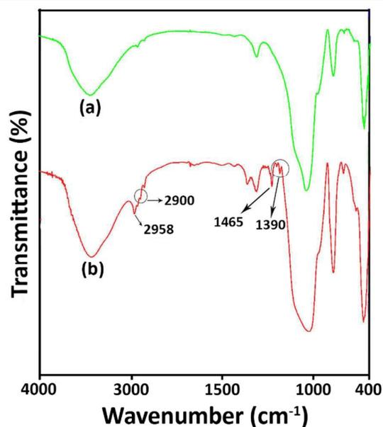
Fig 1. FTIR spectra of SiO<sub>2</sub> (a) and DABCO@SiO<sub>2</sub> (b).
