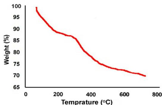
Fig 5. TGA analysis of the catalyst A.
