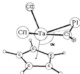
Figure 2. Calculated lowest energy geometry for complex **A**. Selected bond lengths [Å] and angles [°]: P1–Cl1 1.672, P1–Ta 2.486, Cl1–Ta 2.086, Ta–Cl1 2.339, Ta–Cl2 2.337, Cl1–H1 1.099;  $\alpha = 114.8$ , P1–Cl1–H1 135.73.
