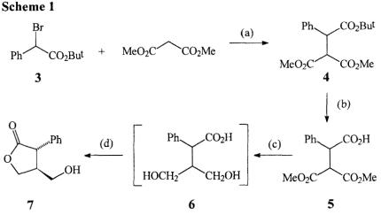
(a): NaOMe/MeOH, reflux 1.5 h, 84%; (b): TFA, r. t., 1 h, 99%; (c): LiBH<sub>4</sub>, ethyl ether, r. t., 5 h; (d): 1 N HCl, 15 min, 83% from 5.
