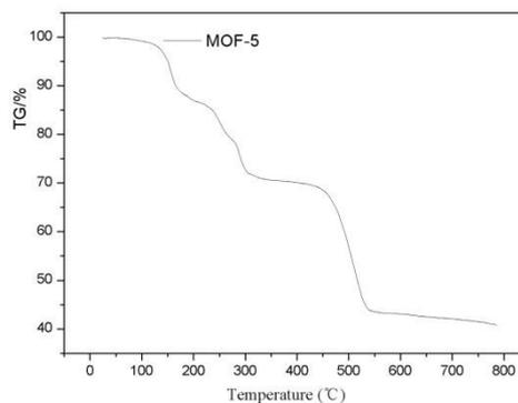
**Fig. 2** Thermogram of MOF-5.
