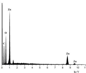
Fig. 6 EDS spectrum of MOF-5.
