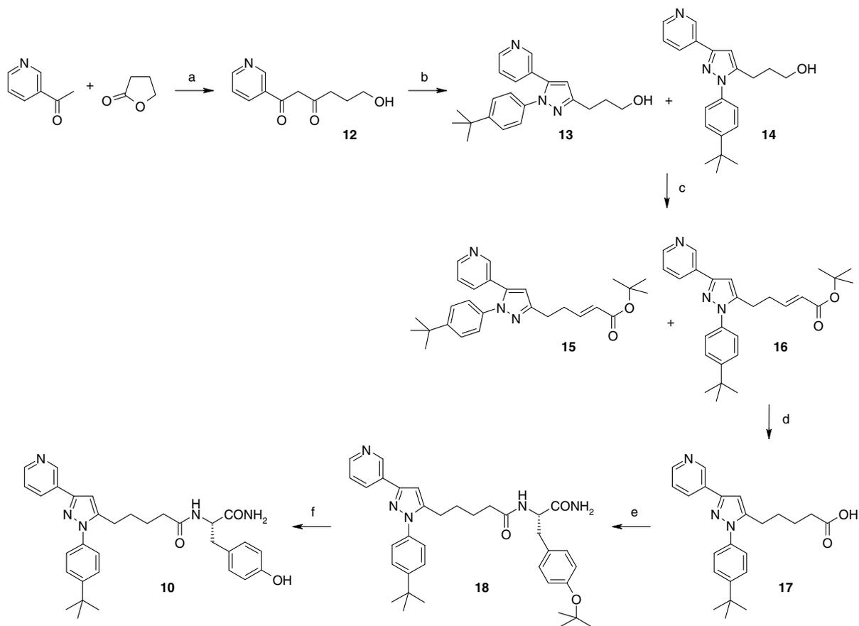
**Scheme 2.** Solution-phase synthesis of pyrazoles. Reagents and conditions: (a) NaH, THF/DMSO, 25 °C, 24 h, 65%; (b)  $p$ -*t*-BuPhNHNH<sub>2</sub>·HCl, 2 M HCl in ether, MeOH, 25 °C, 15 h, 87%; (c) i—Dess–Martin, DCM, 25 °C, 4 h, ii—(EtO)<sub>2</sub>POCH<sub>2</sub>COOtBu, NaH, THF, 0 °C, 1 h, 40%; (d) i—HCOONH<sub>4</sub>, 10% Pd/C, MeOH, reflux, 1 h, ii—TFA/DCM, 25 °C, 4 h, 90%; (e) *O*-*tert*-butyltyrosinamide, EDC, HOBT, DIEA, 25 °C, 24 h, 80%; (f) TFA/DCM, 25 °C, 1 h, 82%.
