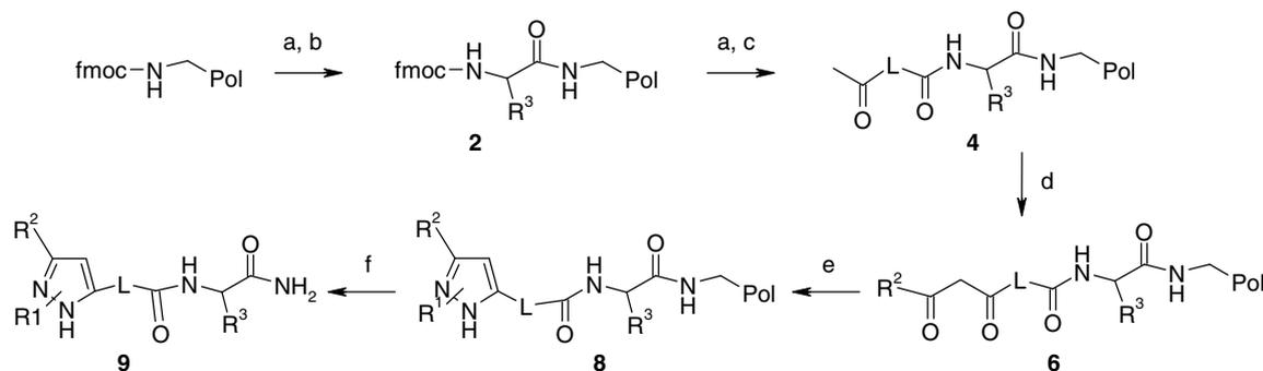
**Scheme 1.** Solid-phase synthesis of pyrazoles. Reagents and conditions: (a) 20% piperidine in DMF, 25 °C, 2 h; (b) HOOCCHR<sub>3</sub>NHFmoc **1**, HATU, DIEA, DMF, 25 °C, 24 h; (c) HOOC-L-COMe **3**, HATU, DIEA, DMF, 25 °C, 24 h; (d) R<sup>2</sup>COOMe **5**, NaH, DMA, 85 °C, 24 h; (e) R<sup>1</sup>NHNH<sub>2</sub> **7**, DIEA, DMA, 80 °C, 24 h; (f) TFA/DCM 2:1, 25 °C, 2 h.
