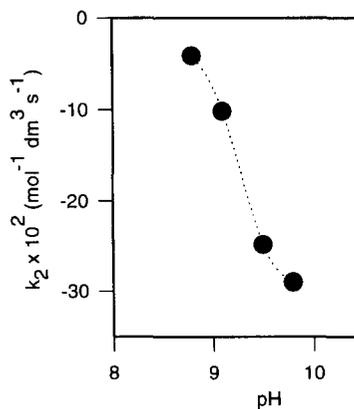
**Figure 4.** Second-order rate constants of *PNPA* hydrolysis as a function of  $pH$  with the  $Zn.D323$  complex.
