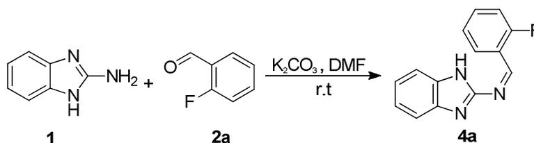
**Scheme 1.** Reaction of 1*H*-benzo[*d*]imidazol-2-amine and 2-fluorobenzaldehyde
