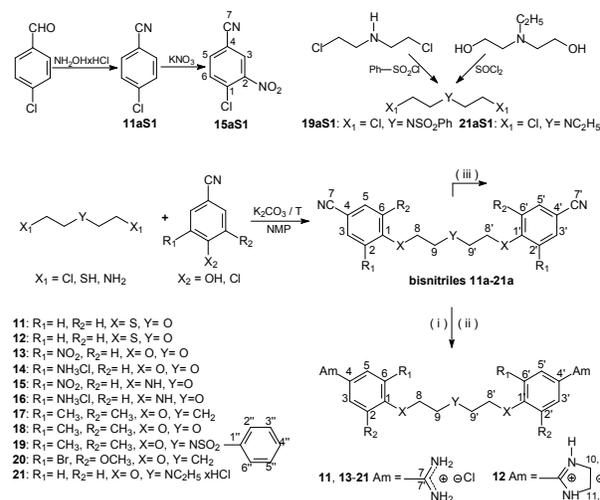
**Scheme 3** Synthetic route to bisamidines **11–21** with atom numbering of the newly synthesized compounds. Reagents and conditions: (i)  $HCl/EtOH$ ; (ii)  $NH_3/EtOH$ , or  $NH_2CH_2CH_2NH_2/EtOH$  in case of **12**; (iii) 1,5-bis(4-cyanophenoxy)-3-oxapentane<sup>33</sup> was treated with  $HNO_3/AC_2O/TFA$  to give **13a**;  $NO_2$  groups in **13a** and **15a** were reduced with  $H_2/Pd$  to obtain **14a** and **16a**.
