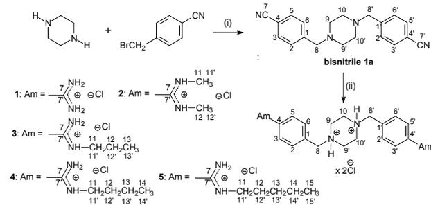
**Scheme 1** Synthetic route to 1,4-bis(methylene)piperazine-linked bisamidines **1–5** with atom numbering of the newly synthesized compounds. Reagents and conditions: (i)  $K_2CO_3$ , DMF; (ii) 1)  $HCl/EtOH$ , 2)  $RNH_2/EtOH$ , 3)  $HCl/EtOH$ .
