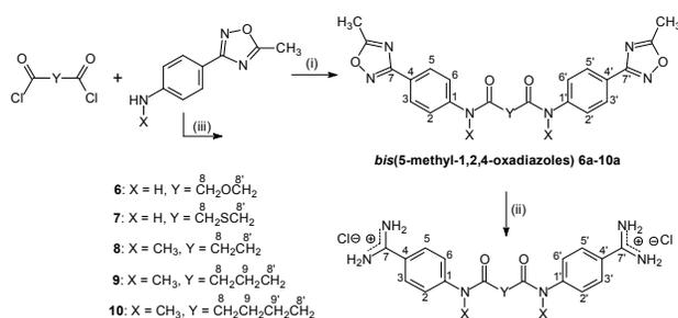
**Scheme 2** Synthetic route to diamide-linked bisamidines **6–10** with atom numbering of the newly synthesized compounds. Reagents and conditions: (i): *N*-methylmorpholine,  $CH_2Cl_2$ ; (ii): 1)  $H_2$ , 10% Pd/C, AcOH, MeOH, 2)  $HCl/MeOH$ ; (iii) 4-(5-methyl-1,2,4-oxadiazol-3-yl)aniline was treated with: 1) paraformaldehyde, MeOH, 2)  $NaBH_4$ , MeOH; to give appropriate *N*-methyl derivative.
