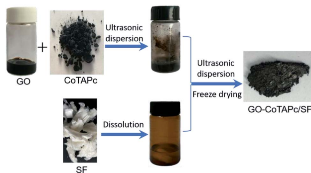
Scheme 1 Illustration for the preparation of GO-CoTAPc/SF gels.
